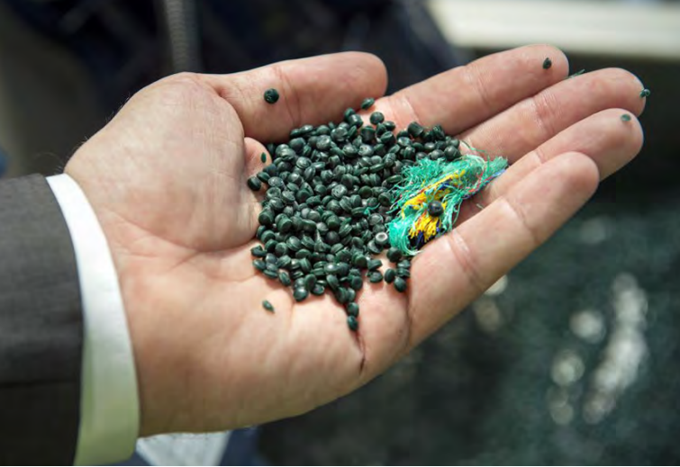
Top and middle left: Plastic fishing nets are recycled to create pellets that BODY BIKE uses in the manufacture of its Smart+ OceanIX model
